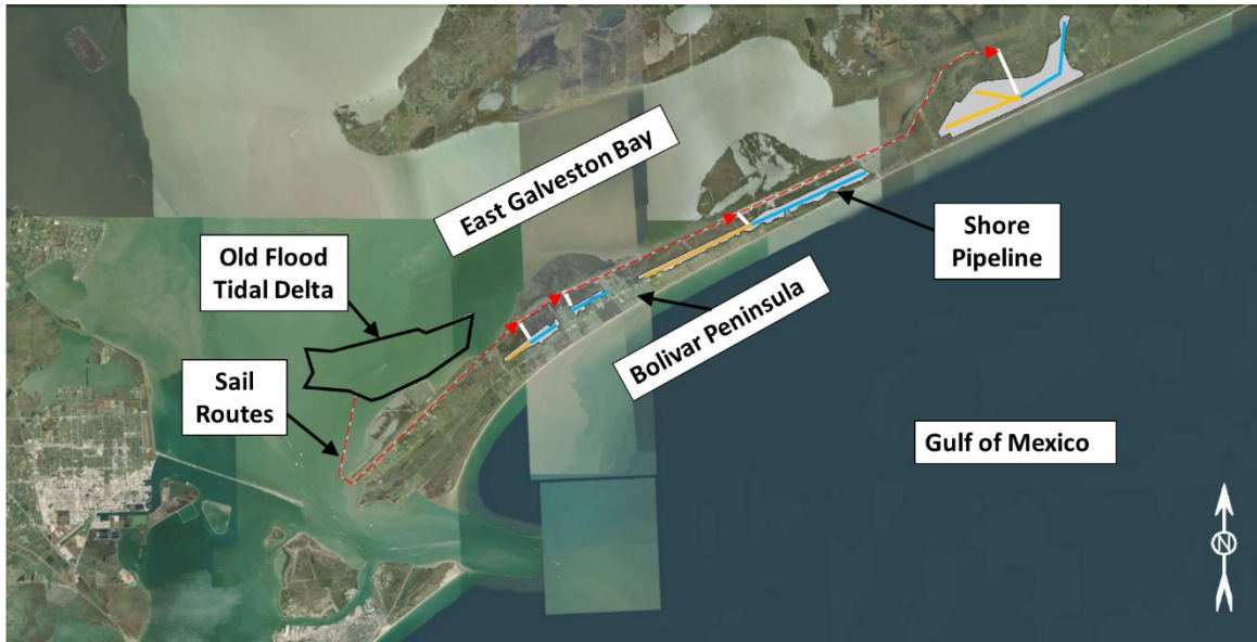
Figure 54. G-28 out-year marsh creation east – East Galveston Bay Tidal Flood Delta Hydraulic dredging to scows
